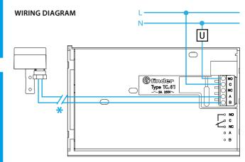
Link terminals A and B of the sensor to terminals A and B of the chronothermostat (maximum cable length: 20 m)
